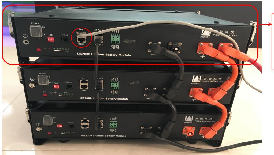
The external communication line should be connected with the module which Link Port 0 is empty(top).
