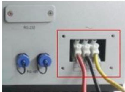
2. Switch off the DC isolator, unplug the DC connectors, then turn on the DC switch to measure the voltage of DC positive to ground and the voltage of DC negative to ground. The reading will be 0 under normal condition, if the voltage is not 0, you can locate the fault area by dividing the voltage by Voc of PV solar module, as in the below example, the Positive to ground voltage is 42V, Negative to ground voltage is 63V, then the fault is located between the 2 and 3 panels.
